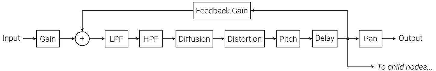
Figure 2: Signal flow for a single delay node.
